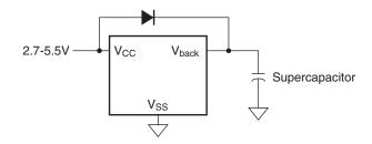
Since the battery switchover occurs at Vcc = Vback-0.1V (see Figure 16), the battery voltage must always be lower than the Vcc voltage during normal operation or the battery will be drained.
