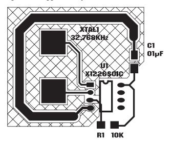
The X1 and X2 connections to the crystal are to be kept as short as possible. A thick ground trace around the crystal is advised to minimize noise intrusion, but ground near the X1 and X2 pins should be avoided as it will add to the load capacitance at those pins. Keep in mind these guidelines for other PCB layers in the vicinity of the RTC device. A small decoupling capacitor at the Vcc pin of the chip is mandatory, with a solid connection to ground.
